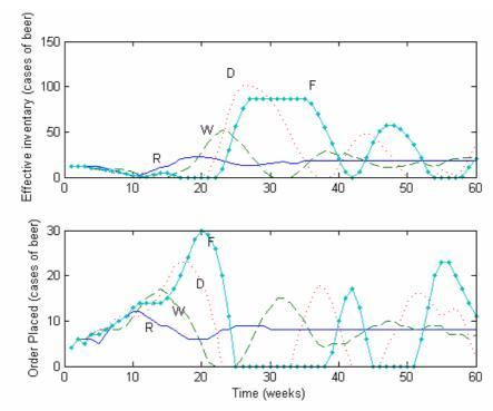
Figure 2. Effective inventory i.e. the number of cases in the stock (upper layer) and order placed (lower layer) of retailer (continuous line), wholesaler (dashed line), distributor (dotted line) and factory (continuous pointed line). Same order policy. Customer demand changes from 4 to 8 cases of beer per week in the fifth week.  $\theta$ = 0.250, Q= 17, optimal parameters:  $\alpha$ <= 0.317 and  $\beta$  = 0.016.
