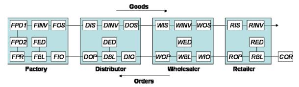
Figure 1. Basic structure of production-distribution system with state variables and orders flow (left arrow) and goods flow (right arrow) in the Beer game model.
